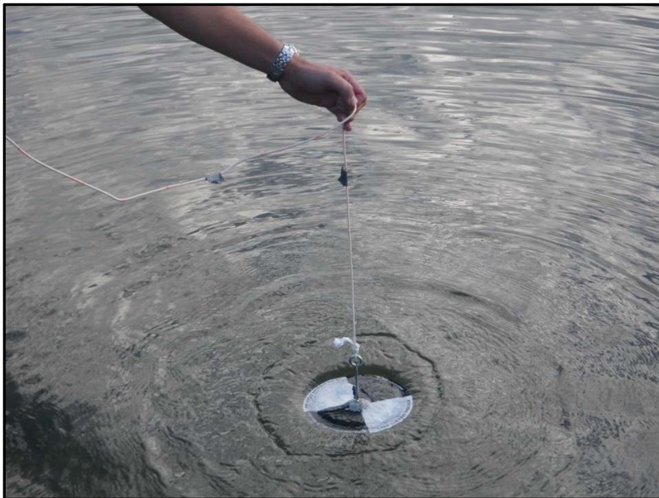
Secchi disc measurement.
